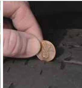
Inadequate Tire Tread
