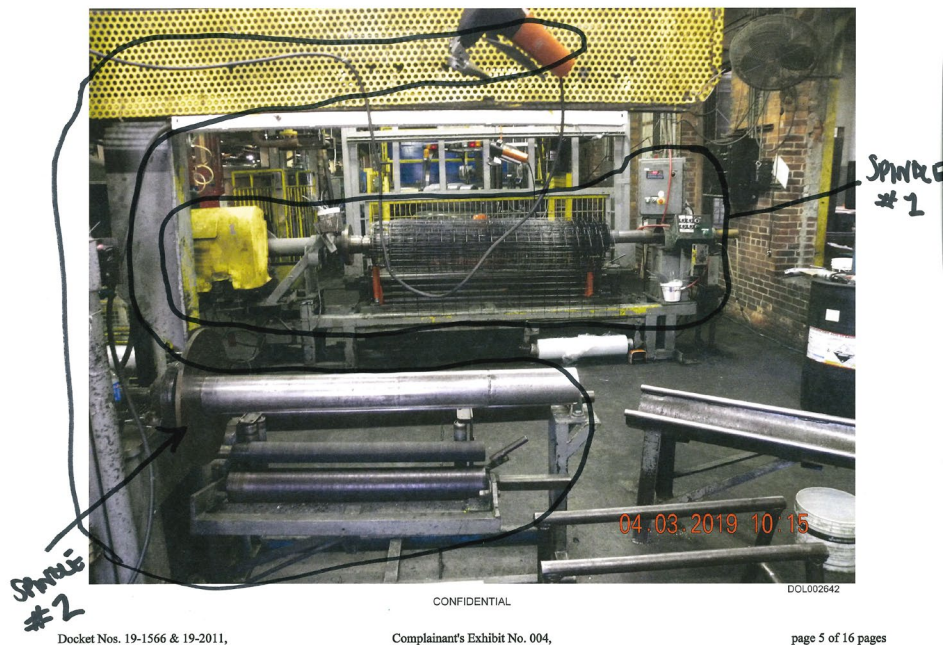
The “Big Spindle” (“Spindle 1”) shown from downstream in the manufacturing process, as it receives mesh from the Main Drive. Vol. 9, C-4 at 5a (annotated at trial); see also Vol. 1, Tr. 109-110. Spindle 2 pictured in the foreground, is not in use. Id. Spindle 3 is not pictured.
