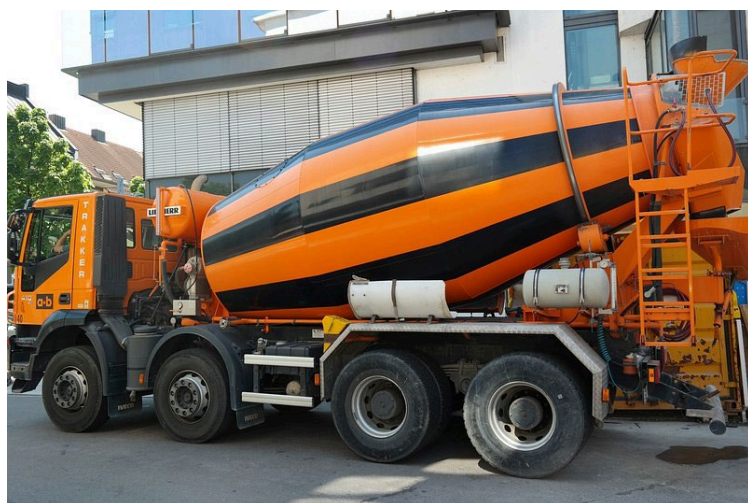
Figure 15. Read-mix concrete truck
