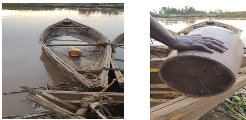
Figure 8. Boat and bucket used in riverbed sand harvesting, Siaya County
