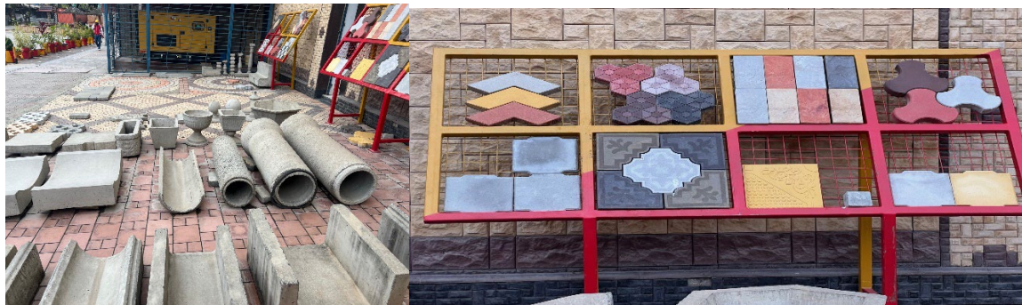
Figure 18. Photos of culverts, roofing tiles, decorative tiles, and paving blocks manufactured with sand
