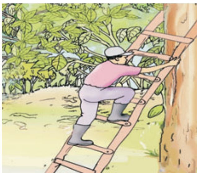
Figure 54: STCP, Always ensure that three parts of your body are in contact with the ladder
