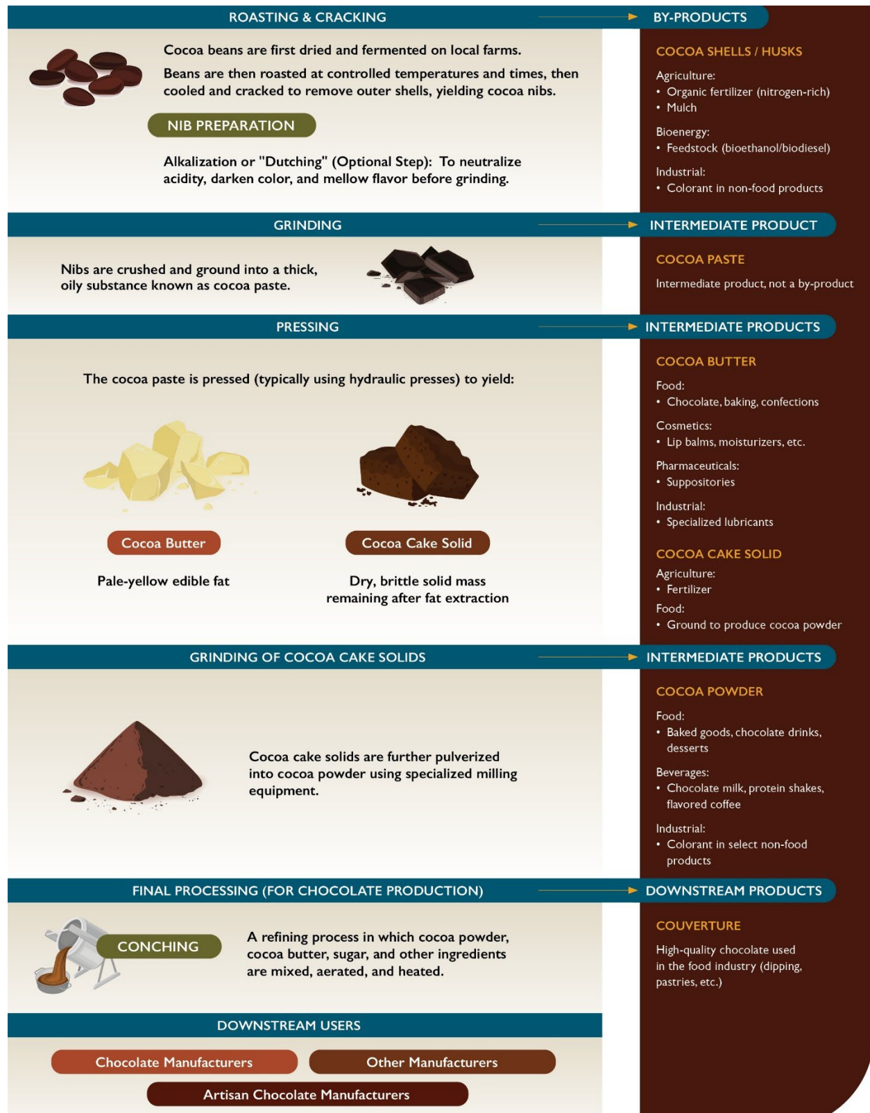
Figure 2. Cocoa processing flowchart
